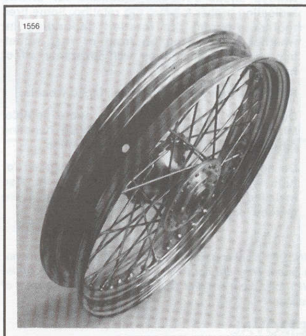
Figure 2-28. Wheel With Rim Strip Installed
